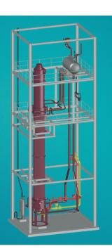
$\ensuremath{\uparrow}$  Layout sketch for a 3 barg HCl gas synthesis unit with steam production
