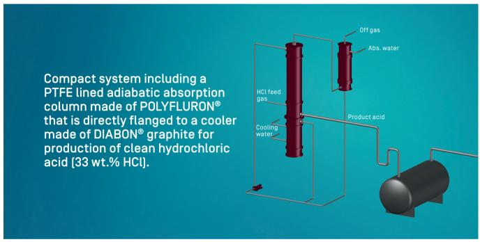
↑ Absorption of HCl gas containing organics and chlorine applying an external cooler
