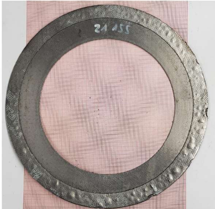
SIGRAFLEX® UNIVERSAL PRO 2 mm V20010C2IP after Fire Test 21-155 according to API Specification 6FB
