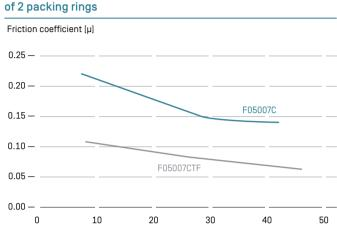
Friction coefficient of SIGRAFLEX foil type TF packing rings
