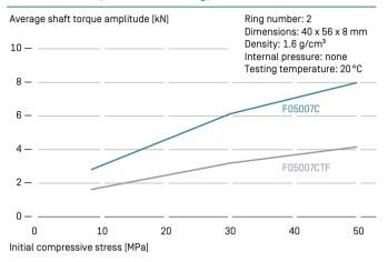
$\uparrow$  Influence of PTFE-coated foil type F05007CTF on the required average shaft torque amplitude in the 5th shaft motion cycle with two installed packing rings, as compared with packings of type F05007C [without PTFE coating].
