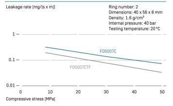
$<sup>\</sup>uparrow$  Comparison between the leakage rates of stuffing box packings in type F05007C [without PTFE coating] and type F05007CTF (with PTFE coating) at 40 bar internal nitrogen pressure and different compressive stresses.
