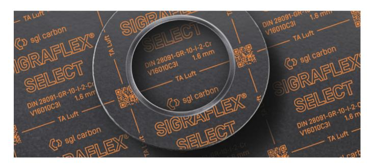
SIGRAFLEX SELECT is a gasket comprised of three SIGRAFLEX flexible graphite foils of various thicknesses reinforced with two 0.05 mm thick stainless steel foils using our proven SIGRAFLEX HOCHDRUCK technology. This gasket has an inner eyelet and is antistick impregnated to reduce leakage and improve handling.
