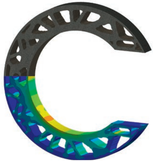
↑ 3D printed optimized cantilever with highest specific stiffness achieved with topology optimization
