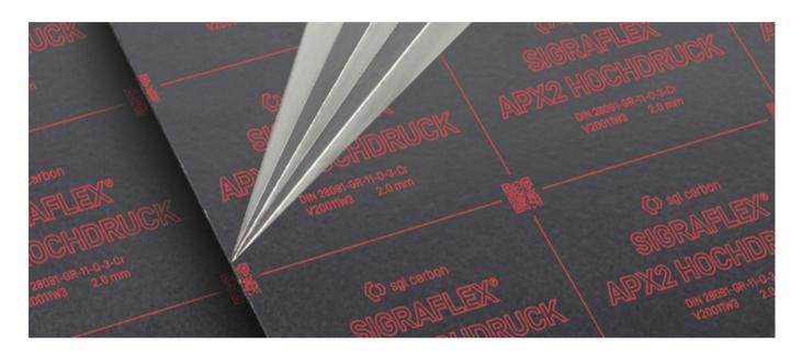
SIGRAFLEX APX2 HOCHDRUCK is a multilayer high-strength gasket sheet – designed for high-temperature applications. It is comprised of 0.5 mm thick layers of highly oxidation resistant SIGRAFLEX APX2 flexible graphite foils and 0.05 mm thick layers of stainless steel foils.
